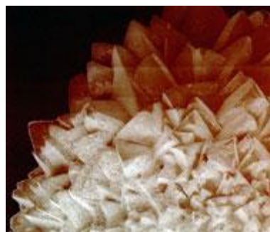
An electron micrograph of calcite crystals in a block of travertine stone. Photo: Eric Doehne.
